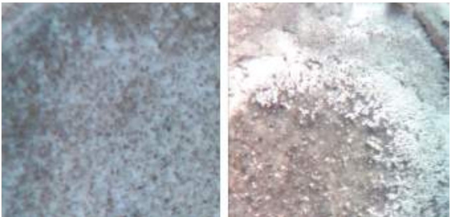
FIGURE 1 - Stereoscopic microscopy images of the surface of cement paste specimens showing CaCO 3 precipitation on the surface. (L) Control - no bacterial treatment (R) treated with one bacterial strain
